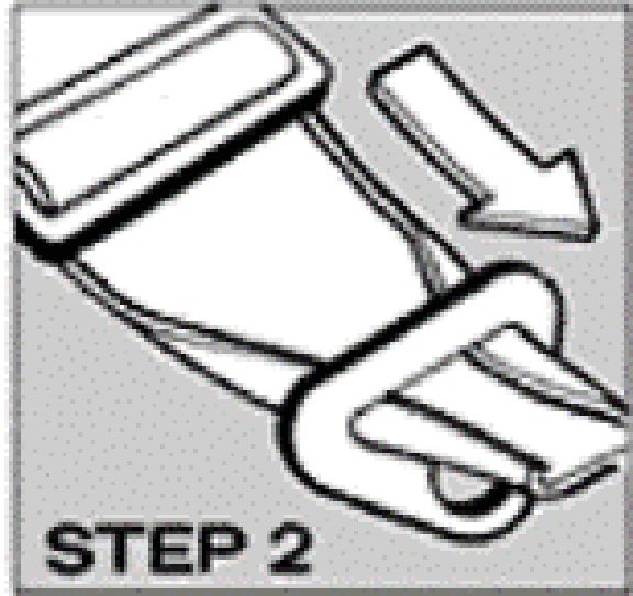
STEP 2: Pull strap to 8" - 10" beyond buckle, fold edges, and insert into mounting bracket.
